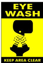
Eyewash stations supply a gentle flood-type spray of tempered water for a minimum of 15 minutes to flush contaminants from the eyes.
